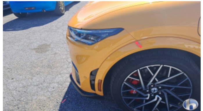
1. Front bumper Chipping from stones - Smart repair
