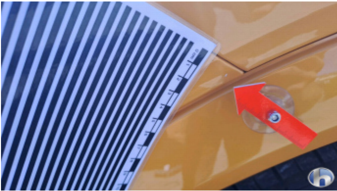
1. Front bumper Chipping from stones - Smart repair
