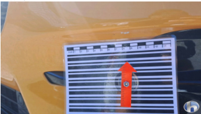
1. Front bumper Chipping from stones - Smart repair
