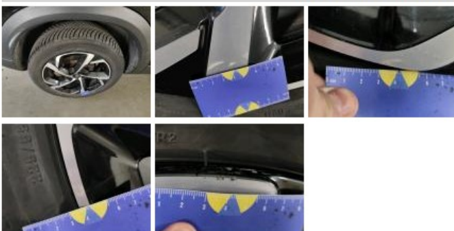
Door FR, Scratch(es), Repair and paint (complete)
