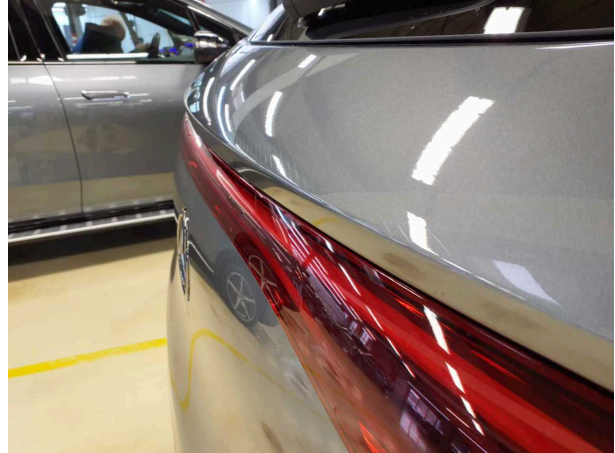
Wear and tear 1: Body: Body (Abrieb (Heckklappe, Heckleuchte re. Stoßstange re.)) - Soiled - Clean
