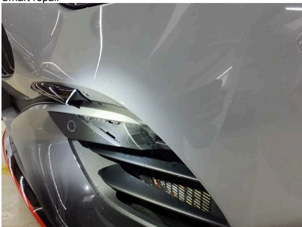
Damage 2: Front bumper: Bumper with Parktronic (Ausbessern) - Abrasion - Smart repair
