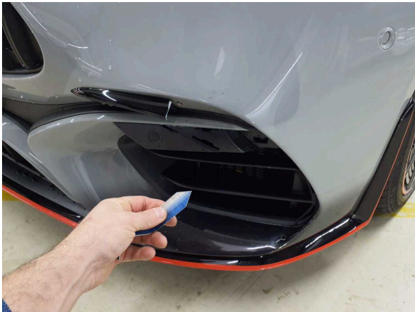
Damage 3: Front bumper: Spoiler - Damaged - Replace
