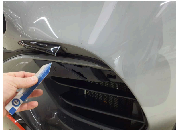
Damage 3: Front bumper: Spoiler - Damaged - Replace
