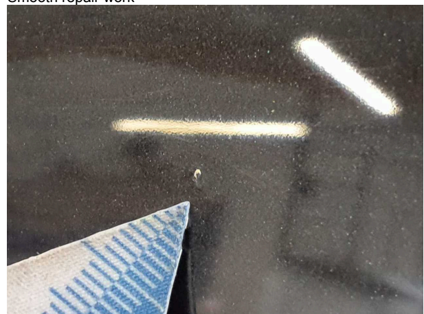
Wear and tear 1: Door - rear left side: Door (Lackeinschlüsse) - Paint defect - No deduction
